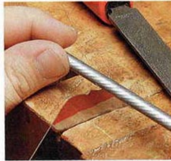
Fine-tune the profile with round and flat files. Finish by honing the edge with stones and burnishing it (for photos of these steps, see Q&A, p. 108).
