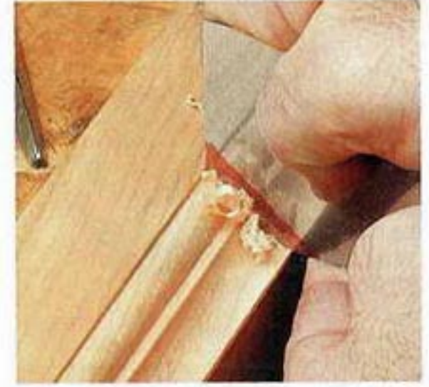
A custom scraper makes short work of tool marks. It would be very difficult to sand this profile, but the scraper smooths the surface and leaves crisp edges.
