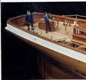
Exact to the nearest detail. Photographs of the actual yacht were used to re-create the captain on the poop deck with a crewman at the wheel. The wheel is made of three layers of apple wood, with turned spokes of apple.
