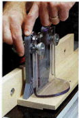
Safety features. A feather-board and blade guard quickly adjust to accommodate various thicknesses of stock.
