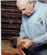
Radius the edge of the stock to the scribe line. Most of the carving is done along this radiused edge.
