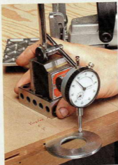
Checking the results. A dial indicator is used to see whether the slot is parallel to the face of the workpiece. A reading of 0.007 in. or less is considered good.
