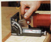
Testing for parallel. For the first test, the adjustable fence supports the joiner (left). The base of the joiner serves as the fence for the second test (right).
