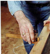
Scribe the carving stock 1/2 in. from the edge. Use straight-grained wood about 1/2 in. thick.
