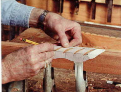
A template made of thin plastic or cardboard simplifies layout. The carving along each apron should begin and end with the same element.
